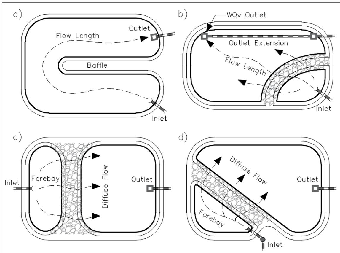
**Figure 2.6.4 Conceptual illustrations of a) an internal baffle, b) the WQv outlet extended to a distant point, c) a forebay baffle to diffuse flow, d) directing the inlet away from the outlet.**
