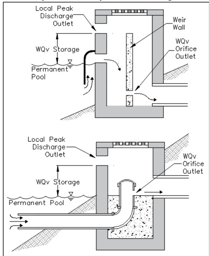
Figure 2.6.2 Conceptual illustrations of small orifice control protection (not to scale).
