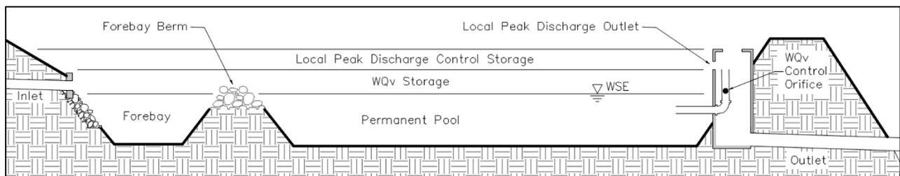
Figure 2.6.1 Typical wet extended detention basin section.
