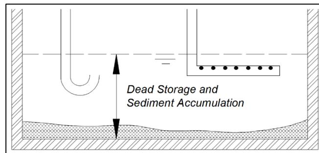
**Figure 2.5.2 Illustration of Two Possible Storage Reservoir Inlet Configurations**
