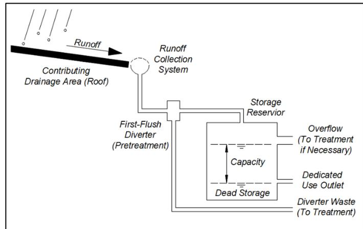
**Figure 2.5.1 Schematic of a Rainwater Harvesting System (after Sample, 2019)**
