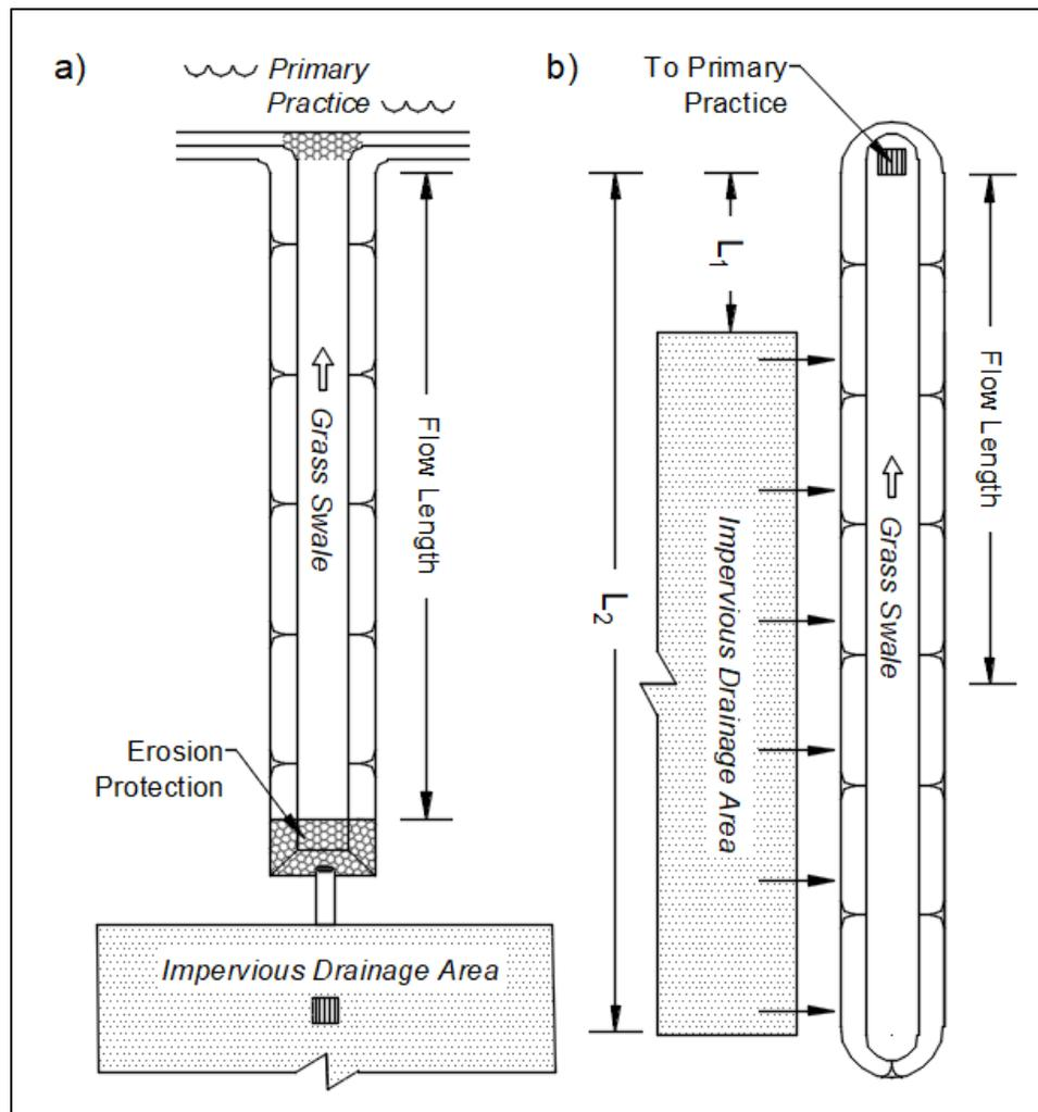
**Figure 2.3.2 a) Flow Entering a Swale at a Defined Point or  $L_{\text{flow}} = L$ , b) Sheet Flow Entering Along the Swale Length Represented as an Average of the Shortest ( $L_1$ ) and Longest ( $L_2$ ) Paths or  $L_{\text{flow}} = (L_1 + L_2) \div 2$**
