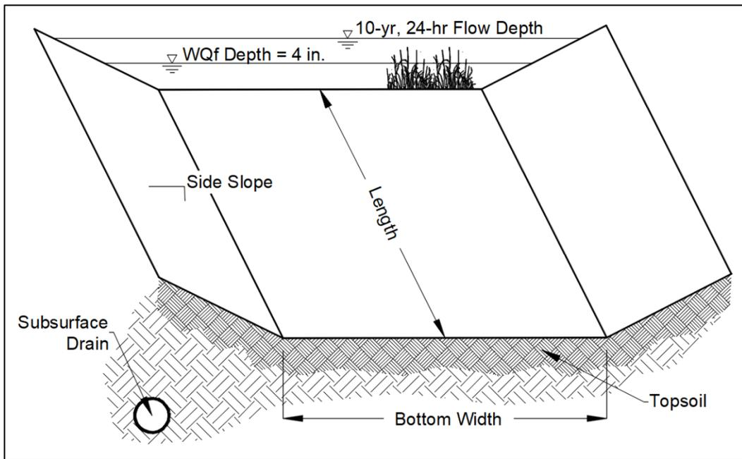
Figure 2.3.1 Grass Swale Geometry and Components
