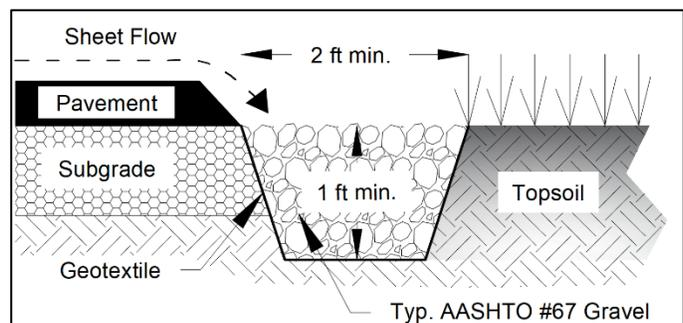
Figure 2.2.2 Typical Gravel Verge/Spreader (not to scale)
