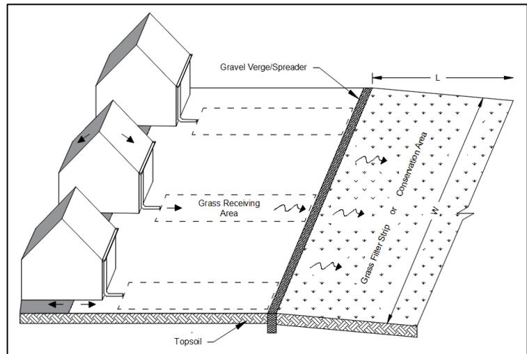
**Figure 2.2.3 Illustration of Impervious Surface Disconnection of Multiple Residential Rear Roofs to Establish Sheet Flow Prior to a Grass Filter Strip or Conservation Area (not to scale)**
