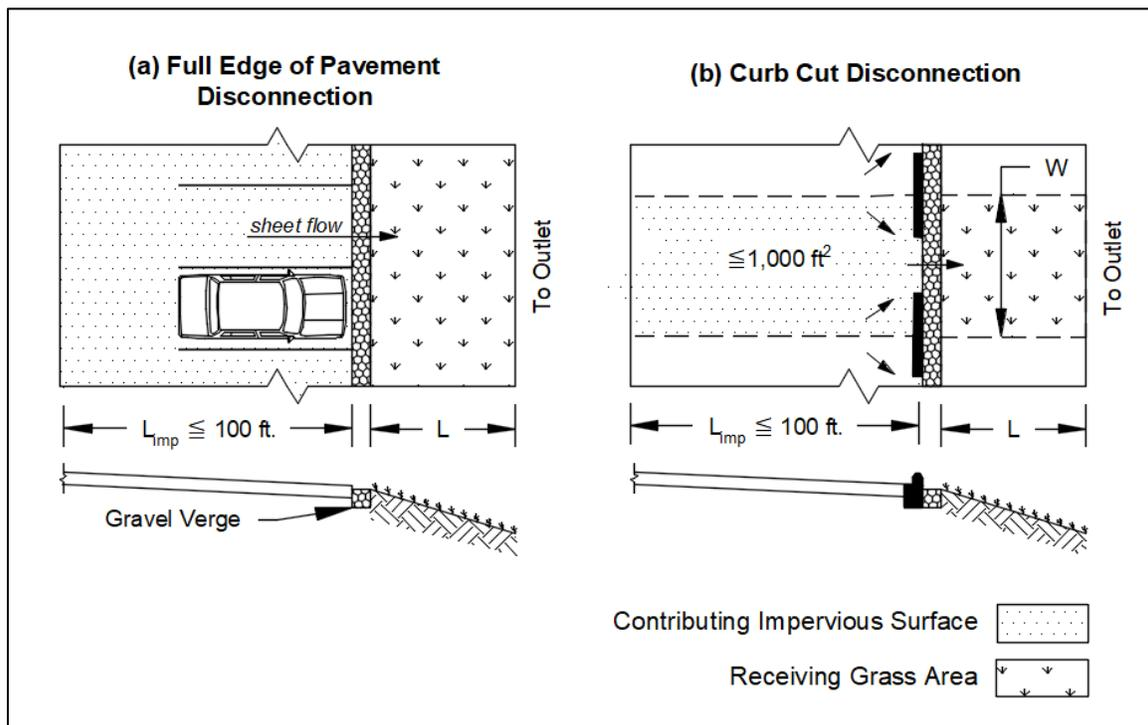
Figure 2.1.1 Illustrations of Pavement Disconnection to a Receiving Grass Area (not to scale)
