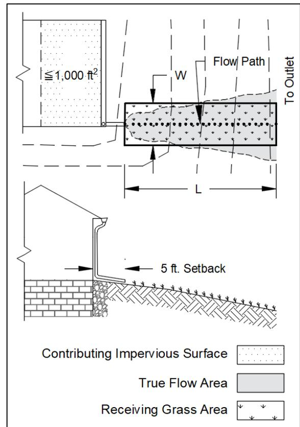
**Figure 2.1.3 Illustration of a Roof Downspout Disconnection to a Receiving Grass Area (not to scale)**
