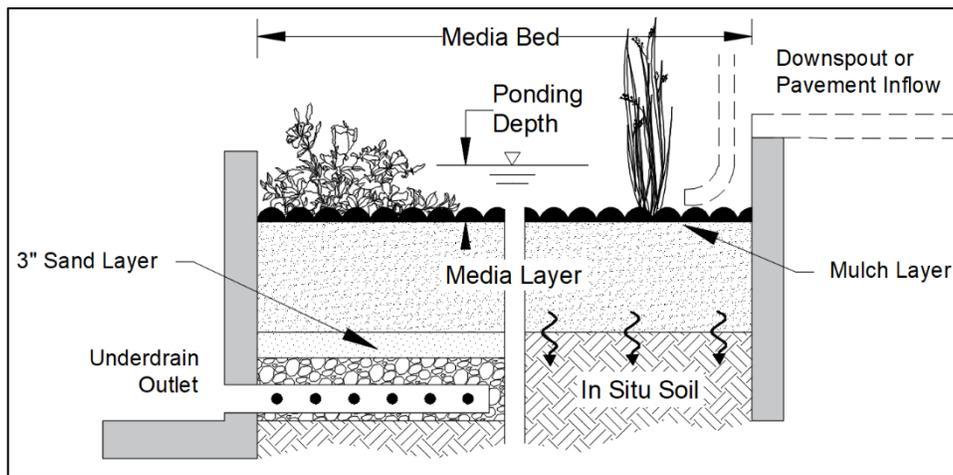
**Figure 2.1.4 Joint Illustration of a Stormwater Planter or Rain Garden with Underdrain to the Left and with Infiltration to the Right (not to scale)**
