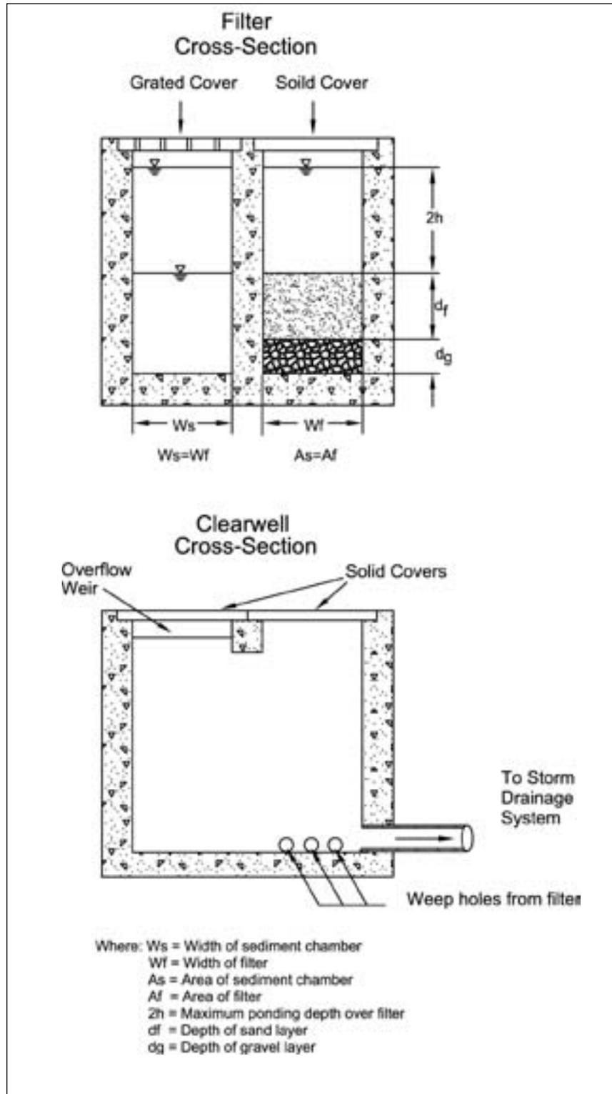
Figure 2.8.5 Delaware filter cross sections.
