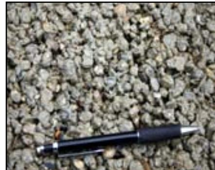
Figure 2.11.6 Pervious Concrete
