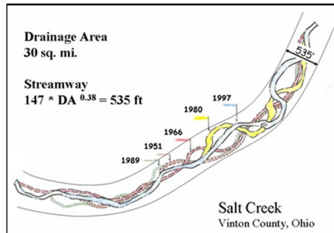
**Figure 1.5.1 An illustration of stream meander migration within a streamway over time (Mecklenburg, D. Ohio Department of Natural Resources).**
