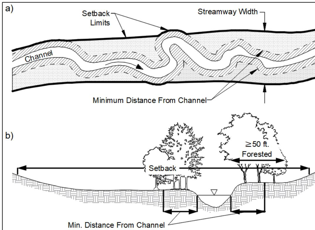
Figure 1.5.2 Illustration of a stream setback in a) plan view and b) section view (not to scale).
