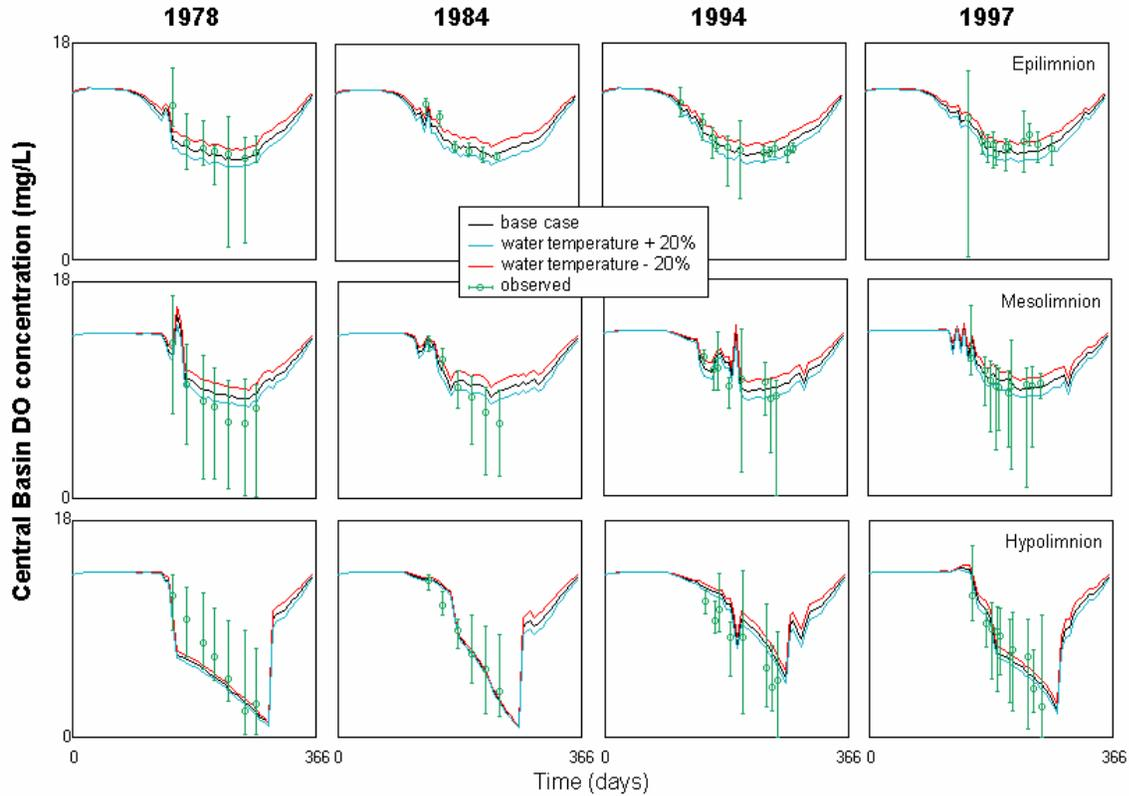
Figure 16b. Lake Erie Central basin DO concentration (base case computed by NWRI Nine-Box Model, with hypothetical changes of water temperature  $\pm 20\%$ , compared to observed means and ranges) for epilimnion, mesolimnion and hypolimnion in 1978, 1984, 1994 and 1997.
