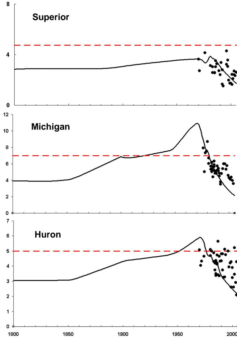
Figure 12. Plots of simulation results and data for TP ( $\mu\text{gP/L}$ ) in the Upper Great Lakes: (a) Superior, (b) Michigan, and (c) Huron. The water-quality objectives are shown as dashed lines.
