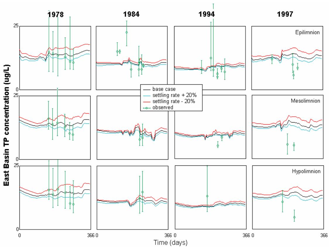
**Figure 16a. Lake Erie East basin TP concentration (base case computed by NWRI Nine-Box Model, with hypothetical changes of settling rate  $\pm 20\%$ , compared to observed means and ranges) for epilimnion, metalimnion and hypolimnion in 1978, 1984, 1994 and 1997.**
