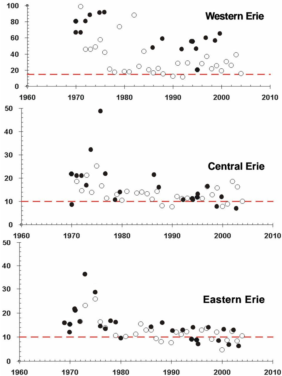
**Figure 3 Mean spring TP concentrations ( $\mu\text{gP/L}$ ) for the offshore waters of the three basins of Lake Erie. The filled and open circles represent Canadian and U.S. data, respectively. Dashed lines represent the target water quality objectives.**
