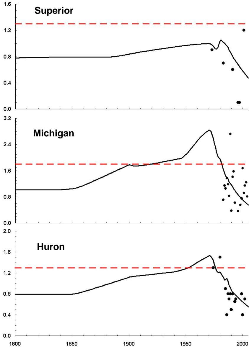
**Figure 13. Plots of simulation results and data for chlorophyll a ( $\mu\text{gP/L}$ ) in the Upper Great Lakes: (a) Superior, (b) Michigan, and (c) Huron. The water-quality objectives are shown as dashed lines.**
