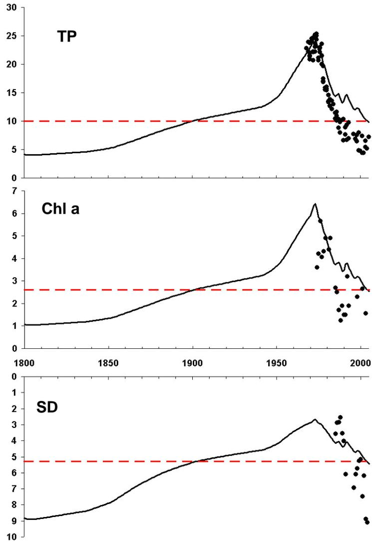
Figure 15. Plots of simulation results and data for (a) TP ( $\mu\text{gP/L}$ ), (b) chlorophyll a ( $\mu\text{gA/L}$ ), and (c) Secchi depth (m) for Lake Ontario. The water-quality objectives are shown as dashed lines.
