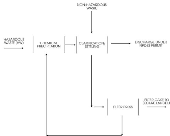
Figure 1. Flow Diagram of a Simple Process System
