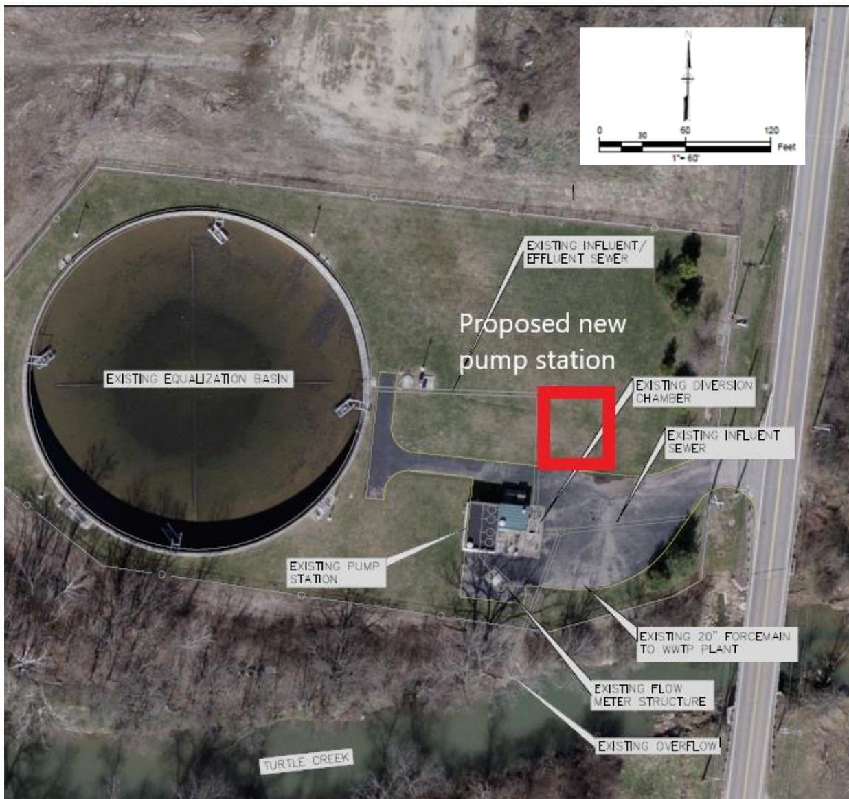
**Figure 3. Map of Glosser Road facility showing existing equalization basin, pump station, and proposed replacement pump station in red**
