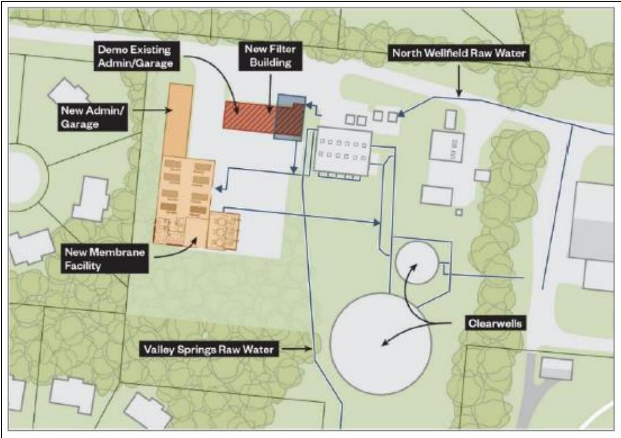
**Figure 5. Drawing of existing NWRWTP showing new building additions to accomplish membrane filtration**
