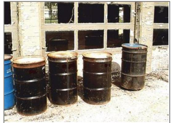
Although these drums are in good condition, they're not labeled with the words "used oil." Make sure your used oil drums are labeled.
