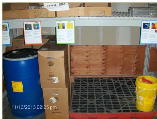
Although the hazardous waste rules do not require generators to provide secondary containment, other rules may apply. This could include containment requirements under Ohio EPA's waste water program or your local sewer ordinance to help prevent spills from entering a sewer system. Contact Ohio EPA's [Division of Surface Water](#) at (614) 644-2001 or check your local sewer ordinance for additional regulations.
