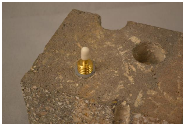
Figure 3. Installed Vapor Pin™
