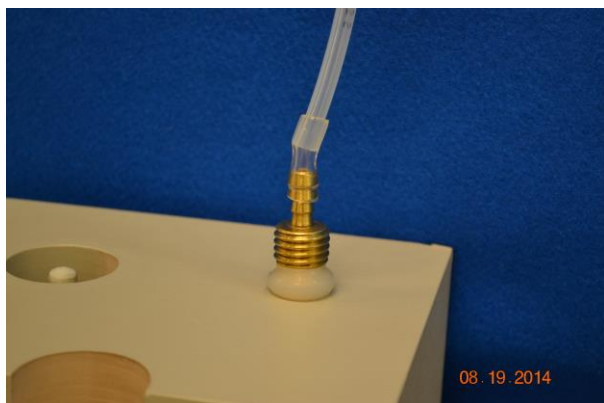
Figure 5. Vapor Pin™ sample connection.
