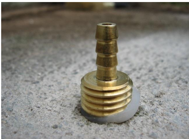
Figure 3: Vapor Pin™ installed and ready for sampling
