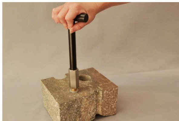
Figure 7. Removing the Vapor Pin™.
