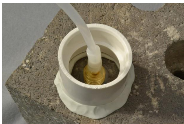
Figure 6. Water dam used for leak detection
