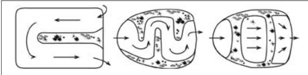
Figure 2.6.1 Flow Routing to Enhance Water Quality Treatment
