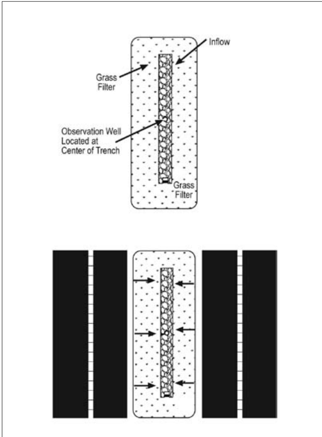
Figure 2.7.3 Illustration of a median strip trench design
