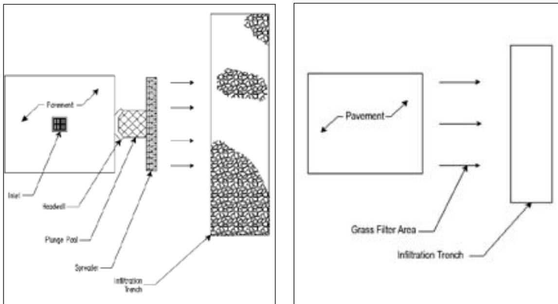
Figure 2.7.2 Typical Infiltration Trench with Plunge Pool
