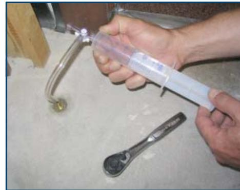
**Subslab soil gas via syringe sampling.**
