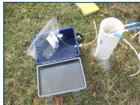
**Exterior soil gas sampling nested vapor points via tedlar bag in a lung box.**
