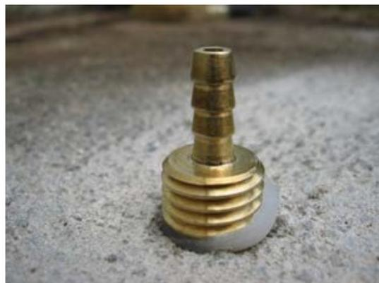
*A close-up view of a sub-slab sample port.*
