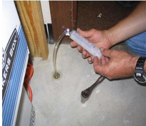
*Collecting a gas sample from a sub-slab sample port.*
