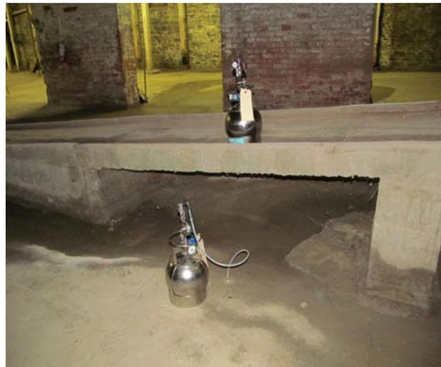
*Collecting an indoor air sample and a sub-slab sample in the basement of a building*
