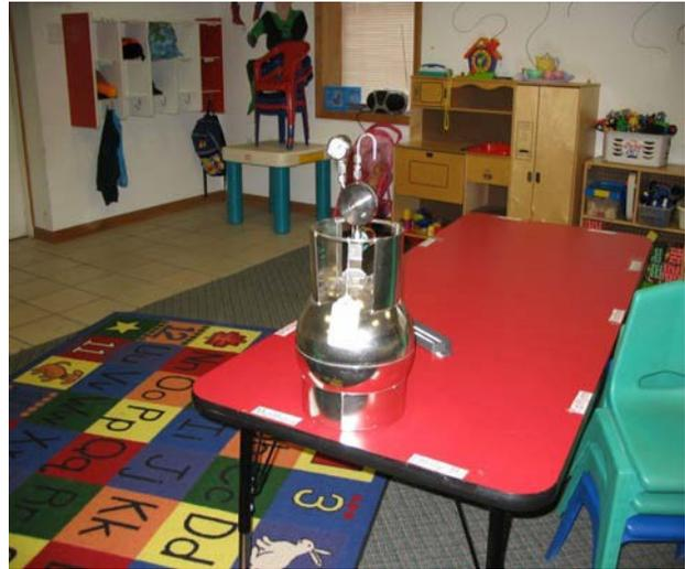
*Sample canister collecting indoor air for analysis.*
