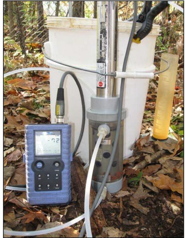
*Water Quality Meter and Flow-through cell.*
