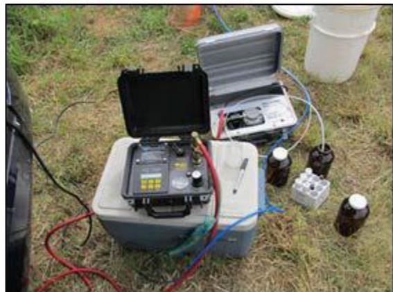
*Compressor and controller for sampling with the bladder pump*
