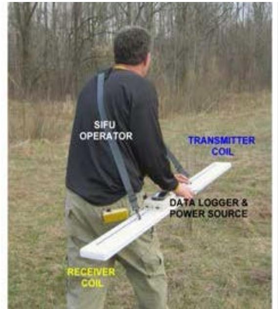
*GEM-2 Electromagnetic Induction Survey in Progress*
