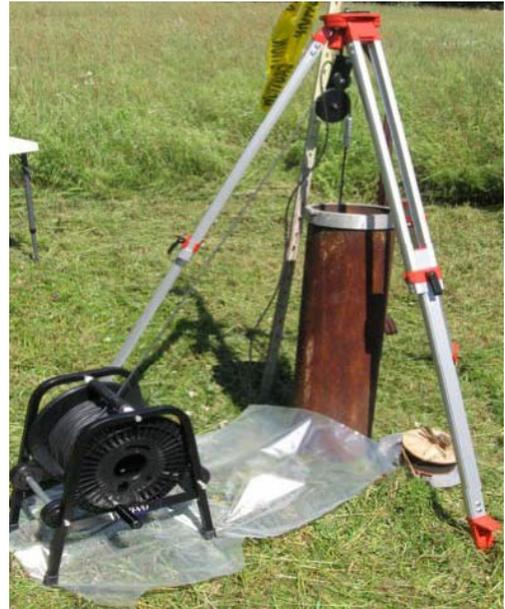
*Well camera and tripod assembly*
