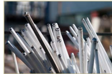
Improper packaging is a common universal waste violation
