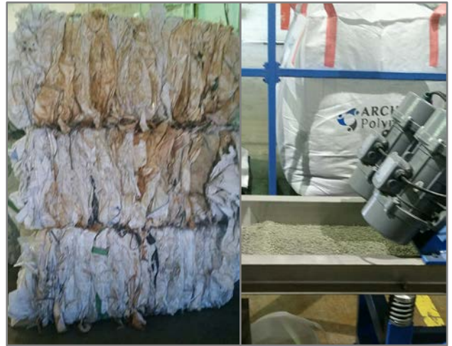
Polypropylene Super Sacks before the recycling process and after as polypropylene pellets for automobile and packaging industries.
